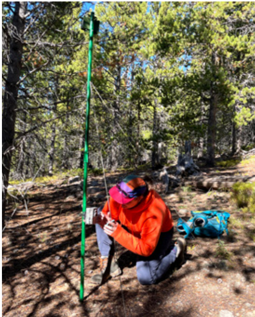
Bat acoustic recording unit with an ultrasonic microphone being deployed in a forested setting. Zack Steel
