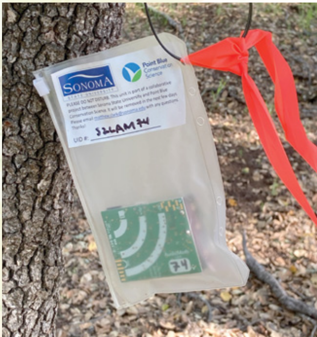
Audiomoth automated sound recording unit (ARU) deployed in an oak woodland to monitor bird sounds as part of the Soundscapes 2 Landscapes program. Point Blue
