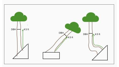
Fig 20. How to locate diameter at breast height (DBH, 4.5 ft) on trees that are not growing straight out of flat ground. Adapted from Dybala (in prep).
