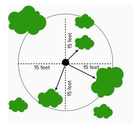
Fig 19. Illustration of the point center quarter method technique. Within each of the quadrants, the closest tree to the point center over 2 inch diameter at breast height is sampled. In this example, sampled trees have an arrow pointing toward them. The tree in the upper left quadrant is not sampled as the trunk falls outside of the circle.
